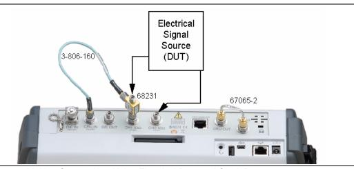
Figure 3-2. Making Connections Using Electrical Data and Clock Recovery.
