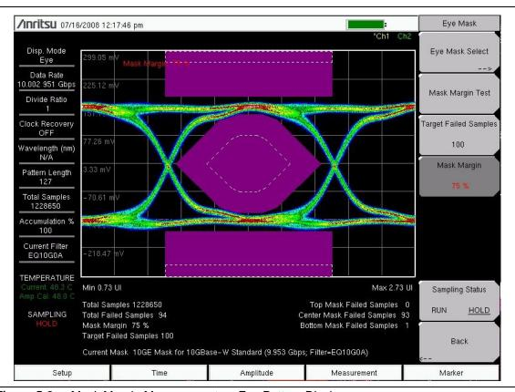
Figure 5-8. Mask Margin Measurement on Eye Pattern Display
