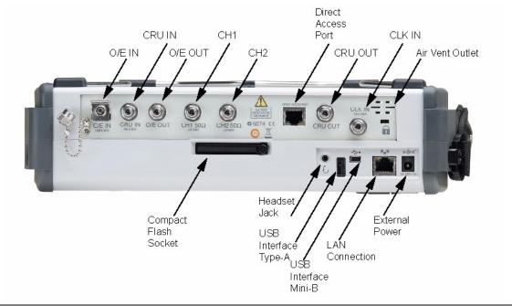
Figure 2-4. Test Panel Connectors
