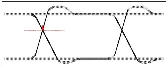
Figure 5-2. Eye Pattern Histograms for Making Jitter Measurements.
