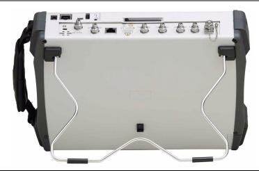
Figure 1-4. Tilt Bail Extended on the Bit Master
