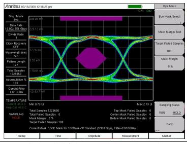
Figure 4-2. Eye pattern display with infinite accumulation and a mask measurement.
