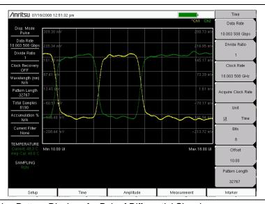
Figure 4-7. Pulse Pattern Display of a Pair of Differential Signals
