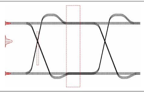
Figure 5-1. Eye Pattern Histograms for Making Statistical Amplitude Measurements
