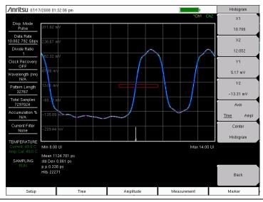
**Figure 4-3.** Pulse pattern display with a histogram measurement.
