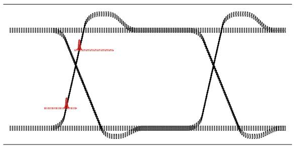
Figure 5-3. Eye Pattern Histograms for Making Rise Time and Fall Time Measurements.
