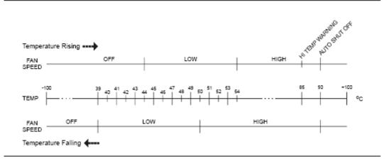
Figure A-1. Fan Speed vs. Temperature
