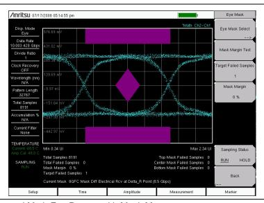
Figure 4-9. Channel Math Eye Pattern with Mask Measurement
