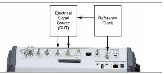
Figure 3-1. Making Connections Using Electrical Data and Electrical Clock
