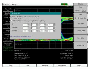
Figure 2-5. IP Address Assigned by Using DHCP
