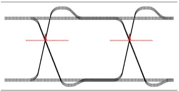
Figure 5-4. Eye pattern histograms for making eye width measurements.
