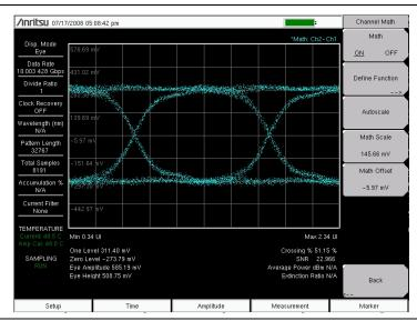
Figure 4-6. Channel Math Result for the Ch2–Ch1 Function
