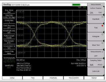
Figure 4-1. Eye pattern measurement display with no accumulation.
