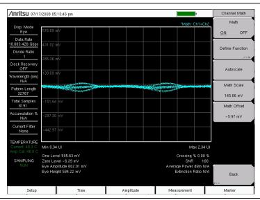
Figure 4-8. Channel Math Eye Pattern for the Ch1+ch2 Function
