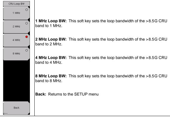
Figure 4-14. CRU Loop BW Submenu
